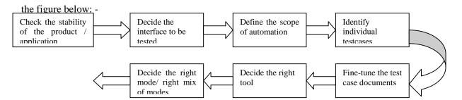
Fig.1: The pre-automation stage cycle
